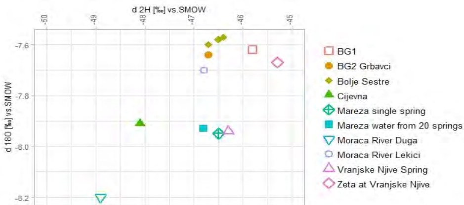
Fig. 9: X-axis shows hydrogen isotope values, Y-axis shows oxygen isotope values, both with respect to VSMOW reference. The Bolje Sestre signatures show the results of 3 different springs in the Bolje Sestre spring pool. The Mareza springs and the Vranjske Njive spring show very similar isotope pattern, distinctively different from the Zeta stream water at Vranjske Njive.
